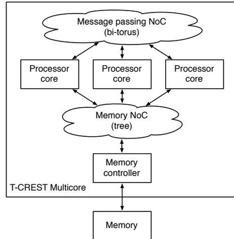
Fig. 1. The T-CREST multicore architecture with several processor cores connected to two NoCs: one for core-to-core message passing and one for access to the shared, external memory
