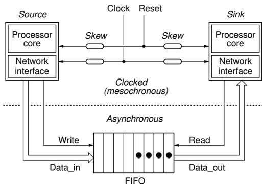
Fig. 2. A model of a virtual circuit connecting two processors. The asynchronous ripple FIFO represents the path through the NoC that packets sent across the virtual circuit follow.
