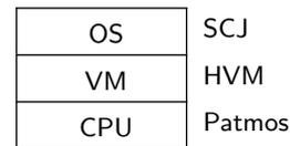
Figure 1: Time-Predictable execution stack for Java.
