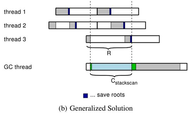
**Figure 3: Visualization of the WCET for root scanning**
