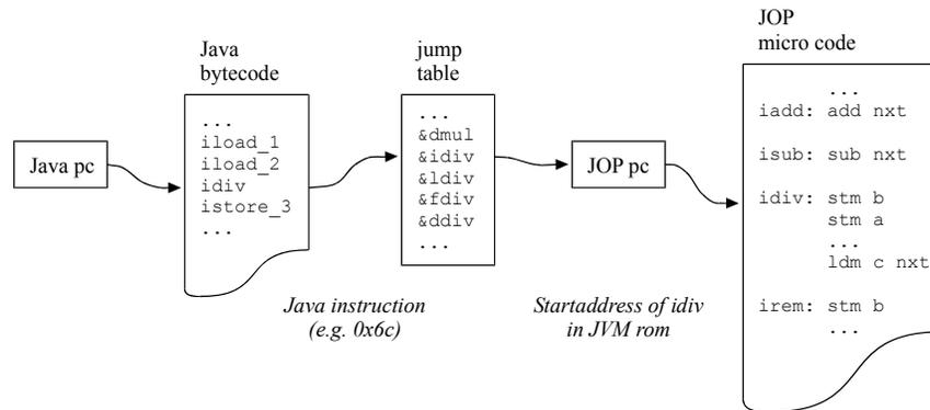
**Fig. 1.** Data flow from the Java program counter to JOP micro code. The fetched bytecode is used as an index into the jump table. The jump table contains the start addresses of the JVM implementation in micro code. This address is loaded into the JOP program counter for every executed bytecode.
