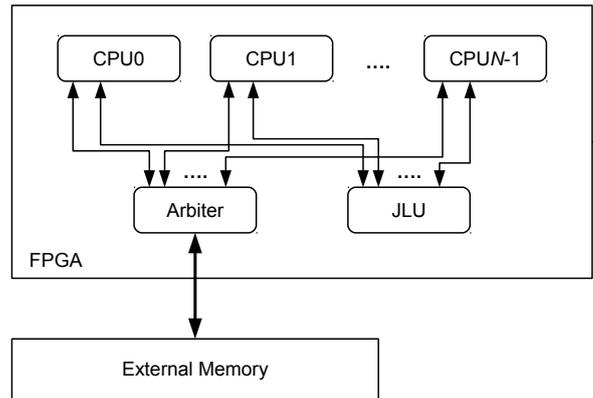
Figure 1: A JOP CMP system with the JLU
