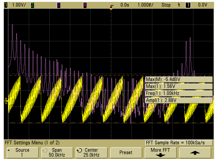
Fig. 2. A 1 kHz Sawtooth signal and the analyzed spectrum up to 50 kHz
