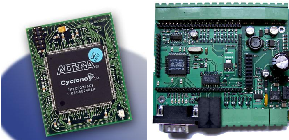
Figure 3.2: The Cyclone EP1C6 FPGA (left) and BaseIO board (right)
