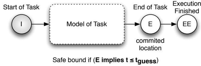
Figure 1. Calculating the WCET bound using UPPAAL
