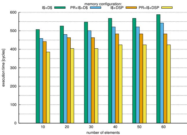
Fig. 5: Binary search algorithm for different memory configurations (I\$: instruction cache, D\$: data cache, PR: prefetcher, DSP: data scratchpad)
